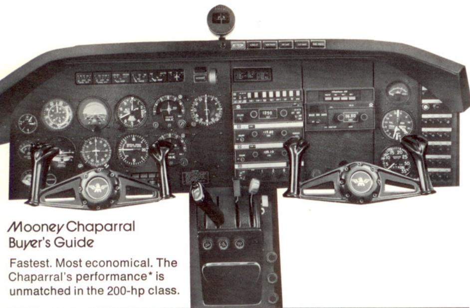
Full flight instrumentation, including pictorial gyros and turn coordinator, are standard. Choose from several radio packages using Narco or King equipment, each clean-room tested and factory installed for reliability.
